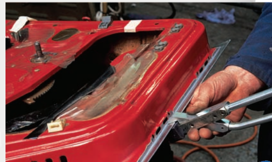
Crimping the panel flange
