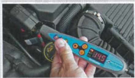
Simple, steady state voltage at the battery – LED display reads volts.
