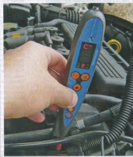
The Terminator is connected to the camshaft sensor. Correct switching is shown by flashing LEDs, while the display shows signal frequency at 7Hz (1 pulse per cycle = 7 \times 2 \times 60 = 840 rpm).
