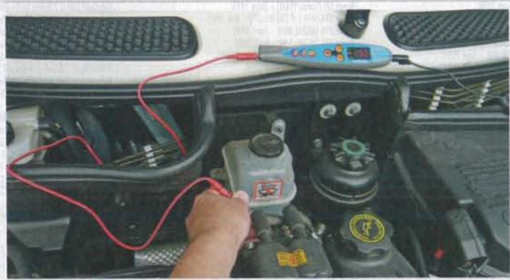
Simple, steady state voltage at the battery – LED display reads volts.
